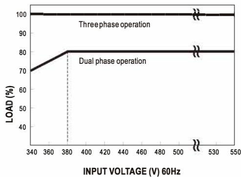
Note : When the dual phase input voltage is between 340~380Vac and ambient temperature is between -10°C~-30°C, the power supply may experience hiccup at cold start. The power supply will start up normally after 5~10 seconds.
