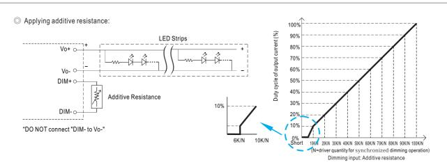
Note: 1. Min. duty cycle of output current is about 6% and the output current is not defined when 0% Iout<6%. 2. The duty cycle of output current could drop down to 0% when dimming input is about 0% or 0%
