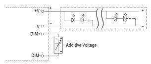
"DO NOT connect "DIM- to -V"
