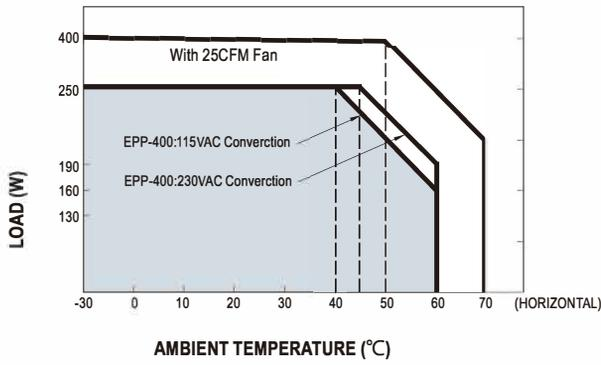
■ **Output Derating VS Input Voltage**
